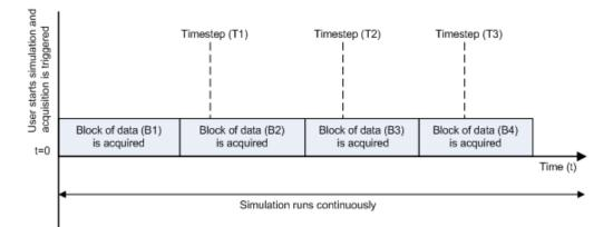
Scenario 2 shows the case when data acquisition speed outpaces simulation speed. At the first time step (T1), the required block of data (B1) has been completely acquired. Therefore, the simulation runs continuously.
