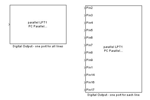
The Digital Output block inherits the sample time from the driving block connected to the input port. The data type of the signal at the input port must be a logical data type.
