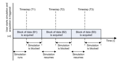
Scenario 1 shows the case when simulation speed outpaces data acquisition speed. At the first time step (T1), the required block of data (B1) is still being acquired. Therefore, the simulation does not continue until B1 is completely acquired.
