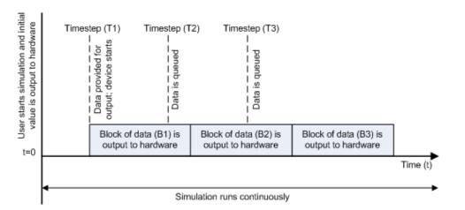
Asynchronous Analog Output – Scenario 2
