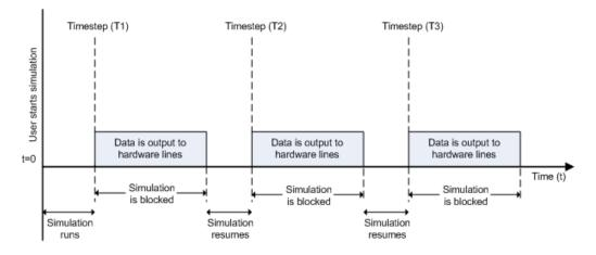
At the first time step (T1), data is output to the selected hardware lines. The simulation does not continue until data is output to all lines.
